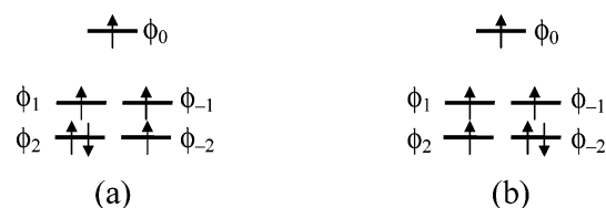
Figure 2. Two low-energy electron configurations expected for a high-spin d^6 ion at a linear two-coordinate site. It is assumed that the high-spin d^6 ion of a transition metal M forms a linear two-coordinate complex \text{ML}_2 with two main group elements L , and the electron configurations are described in terms of the molecular orbitals \phi_n ( n = 0, \pm 1, \pm 2 ) of \text{ML}_2 . The d -orbital of M with magnetic quantum number m_l = n is the major component of the molecular orbital \phi_n , namely, the d_z^2 orbital in \phi_0 and the \{d_{xz}, d_{yz}\} orbitals in the set \{\phi_{+1}, \phi_{-1}\} . In linear \text{ML}_2 the ligand s/p orbitals cannot mix with the \{d_{xy}, d_{x^2-y^2}\} orbitals of M , so that the molecular orbitals \{\phi_{+2}, \phi_{-2}\} are composed solely of the \{d_{xy}, d_{x^2-y^2}\} orbitals.
